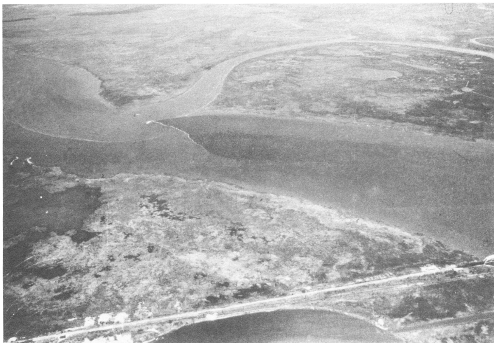
Figure 11. Mouth of the Pearl River at the Rigolets. Dark Colored Water is a Wedge of Saline Water Being Pushed in by an Incoming Tide. Station WURL-1 is in Upper Right.
