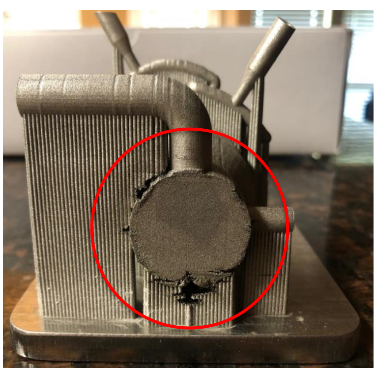
First test print w/ failure due to damaged wiper blade
