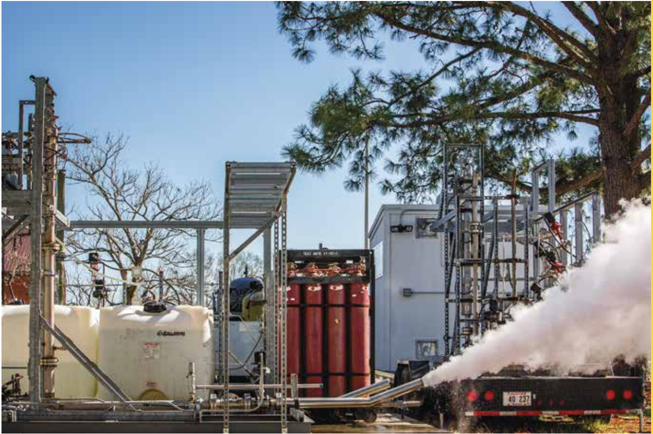
Dandina Rao's Gas-Assisted Gravity Drainage, or GAGD, process demonstrated at the LSU Innovation Park. Photo by LSU.
