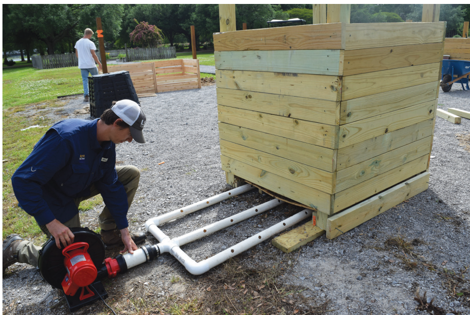
LSU AgCenter Extension Agent Bert Hammett inserts an aeration system into a composting bin at the new teaching compost facility.
